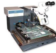
DRS25 Semi-Automated and Repeatable Thermal Performance with Highly Accurate Vision Alignment.
