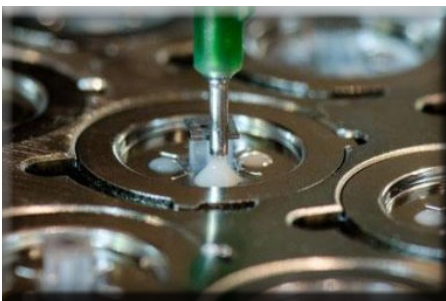
Precise Process Control - Automatic Needle Calibrations, Cleaning Stations, and Dispense Parameter Adjustments.
